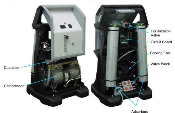
Figure 4-2 Internal Components (Typical Oxygen Generator)
