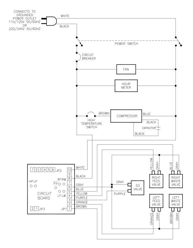
Figure A-4: Electrical Schematic
