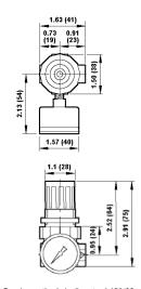
Panel mounting hole diameter 1.19" (30 mm) Maximum panel thickness 0.25" (6 mm)
