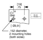
▲ CAUTION: Be sure mounting screws do not penetrate yoke far enough to damage coil.
