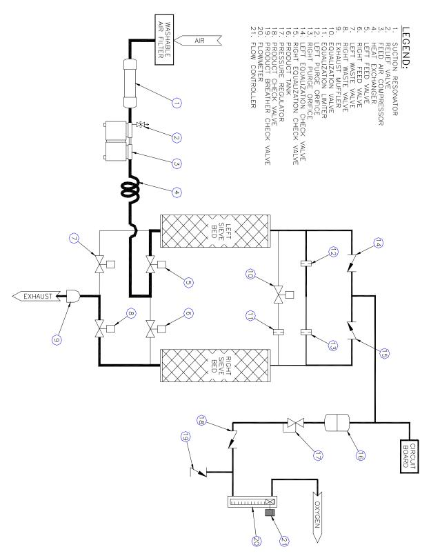
Figure A-2: Onyx+ Flow Schematic
