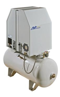
Specifically designed for reliability, energy efficiency, and ease-of-use, there are thousands of Topaz PSA Oxygen Generators currently in use throughout the world. Generating up to 18 LPM (38 SCFH) in a compact package, at up to 95.5% oxygen concentration, the Dual Topaz Plus is a great fit for a wide range of commercial applications.
