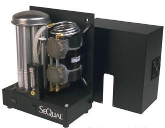
The Workhorse-23 Profile is a revolutionary oxygen concentrator system that provides 23 SCFH (0.60 Nm³/hr or 10.8 LPM) of oxygen (including an oil-less compressor on-board) in the same space as the previous generation conventional two-bed 12 SCFH (0.31 Nm³/hr or 5.7 LPM) or 15 SCFH (0.39 Nm³/hr or 7.1 LPM) systems.
