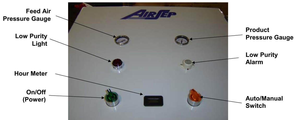
Figure 4.2: PSA Enclosure Controls and Indicators
