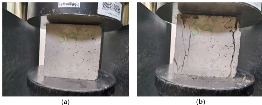
Figure 11. Concrete with ordinary tap water before (a) and after compressive strength testing (b) following 150 F-T cycles.
