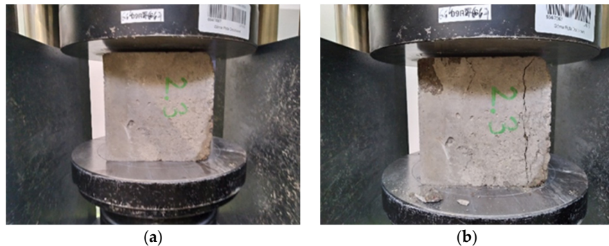
Figure 10. Concrete with micro-nano ozone bubbles before (a) and after compressive strength testing (b) following 150 F-T cycles.
