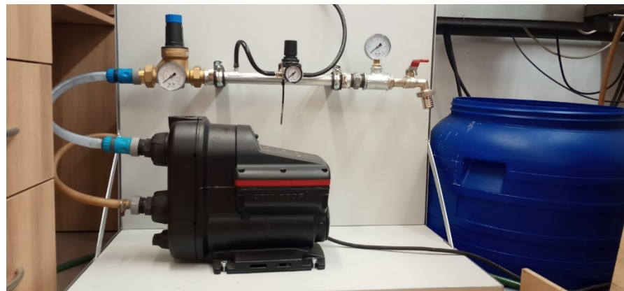
Figure 3. Water generator with micro-nano gas bubbles under laboratory conditions.
