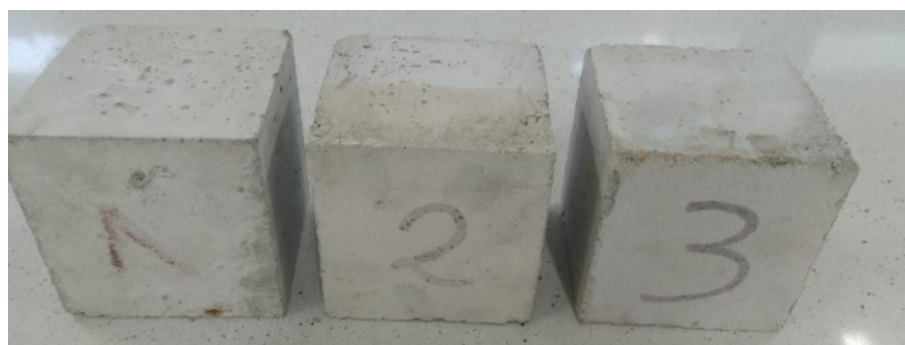
Figure 1. Concretes produced: (1) concrete with micro-nano oxygen bubbles; (2) concrete with micro-nano ozone bubbles; (3) references concrete.
