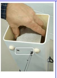
3. Using side cutters or strong scissors clip the cable ties that hold the tubes in place and remove the ties.
