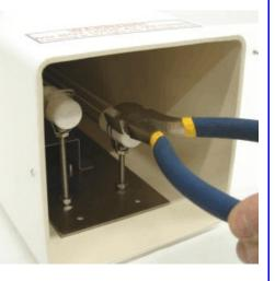
4. To remove the tube lift the end up out of the stainless support and pull while wiggling the tube back and forth being careful not to break it on the steel supports.
