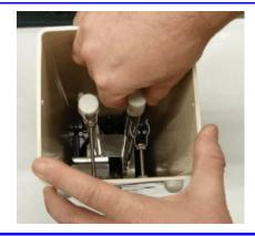
5.Take all the tubes and use an alcohol moistened paper towel or a lightly soap and water moistened paper towel to wipe the tubes down and remove any deposits. If soap water is used then a second wiping with a clean water moistened paper towel will be required to remove the soap.
