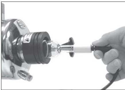
Step 3 – Withdraw Lamp
