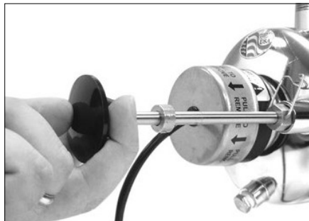
Step 2 – Gently pull wiper knob out
