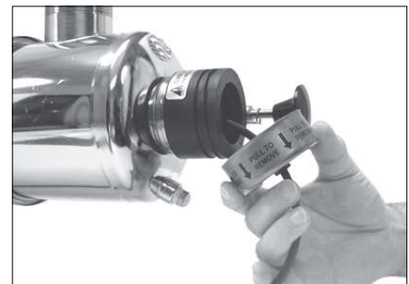
Step 2 – Remove End Cap
